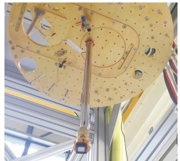
Paragraf cryogenic GHS mounted on an Oxford Instrument's Proteox dilution refrigerator
