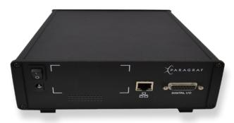
Paragraf's Multi Sensor Test Unit provides a self-contained, turn-key solution for the easy configuration and operation of up to four Graphene Hall Sensors (GHS) for a wide range of applications.
